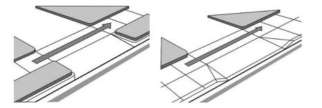
The goal of this plan is to maximize the level area of the driveway and to minimize the sloped area and align it with the parkway, unless the sidewalk is 10' wide or narrower. Image source: ITE Designing Walkable Urban Thoroughfares: A Context Sensitive Approach at ITE.com.
