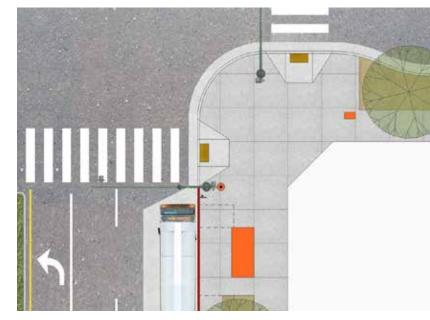
Plan view of directional ramps at a curb extension.
