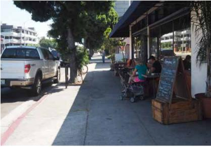
West of Centinela Avenue sidewalks are generally narrower, ranging from 8' to 23' wide. Buildings are typically setback a few feet even on narrow sidewalks, so there is room for a narrow row of tables.
