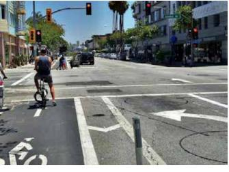
**Top:** On Reseda Blvd. the cycle track is dropped at intersections and bikes and cars share a "mixing zone." Middle: Alternatively, the cycle track could continue to the intersection, where protection is most critical, with the addition of a protected pedestrian/bike signal cycle as in Long Beach.
