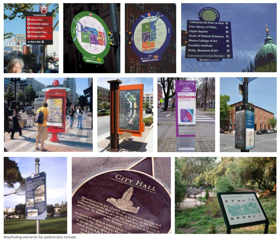
**Top row**: directional signs typically mounted on street light poles **Middle row**: maps, either mounted on street light poles or freestanding Bottom row: interpretive signs pole-mounted upright, embedded in pavement or low-profile for easier reading by everyone.
