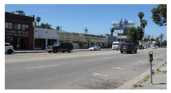
The roadway is typically 70 feet wide with two travel lanes and full-time on-street parking in each direction with a continuous center turn lane, which can accommodate medians in some midblock locations. Buildings are typically one or two story commercial storefronts with entrances along the sidewalk and limited parking behind. Some segments have more street trees than others.
