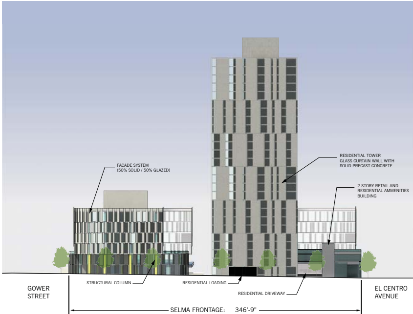
SELMA STREET ELEVATION [NORTH]
