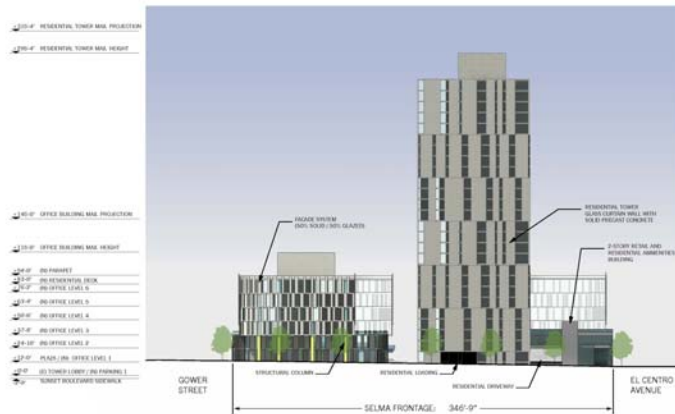
SELMA STREET ELEVATION [NORTH]
