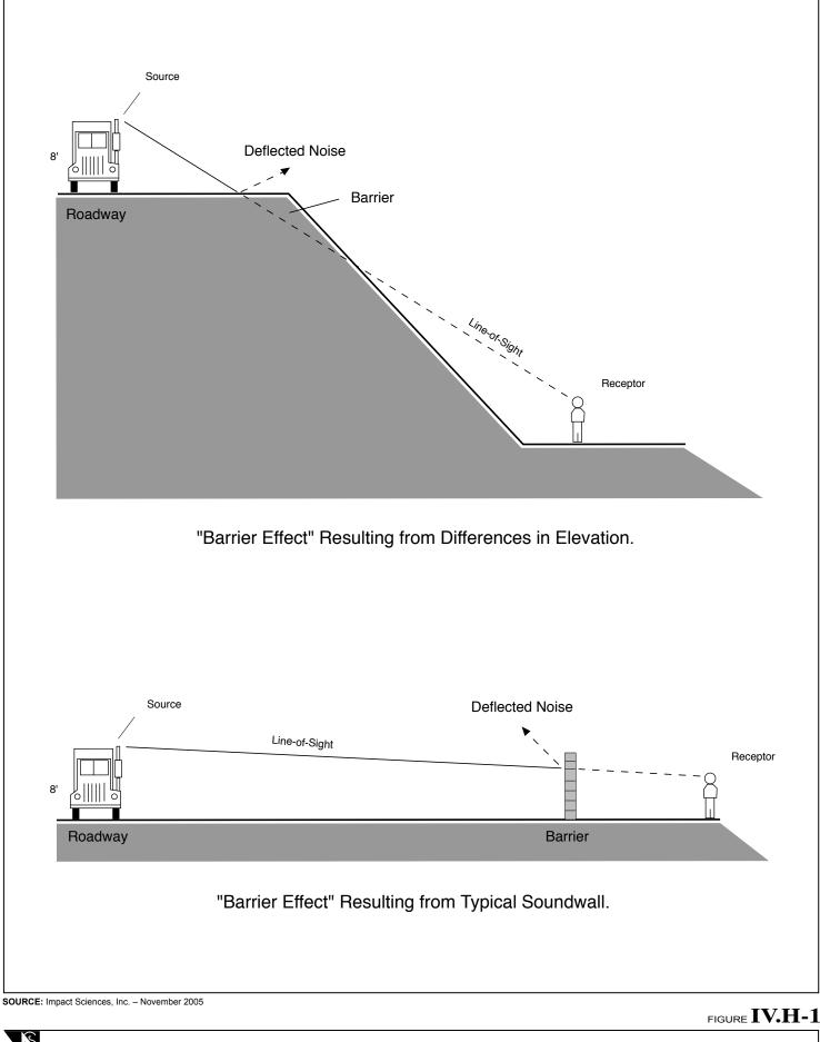
Noise Attenuation by Barriers and Elevation Differences
