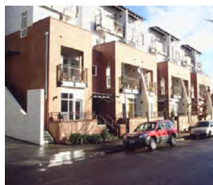
Guideline 2c example. Entrances should be slightly set back from the property line and elevated two to five feet. Step backs can be incorporated to provide balcony and terrace spaces.
