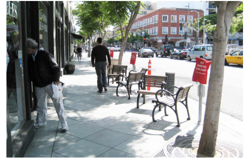
Street furniture, trees, and other amenities can provide a buffer zone between pedestrians, vehicular traffic, and other modes of transportation. (Figure A.4.o)
