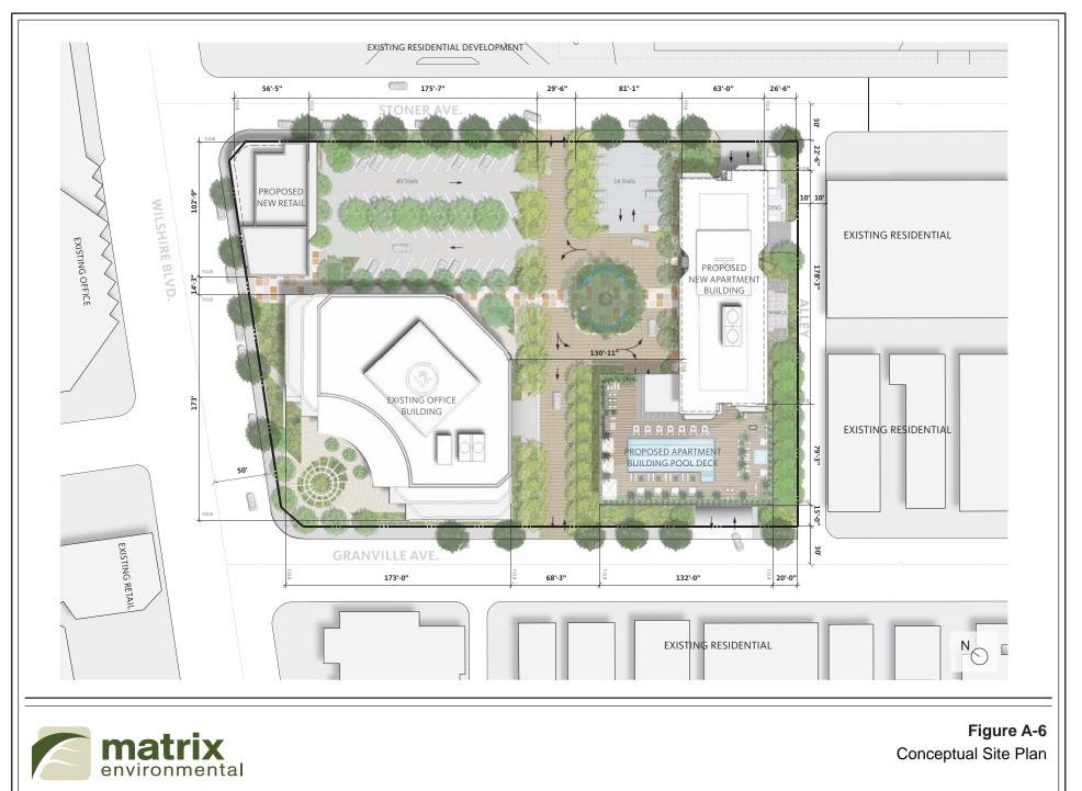
structures.<sup>2</sup> As shown in Figure A-6 on page A-11, an outdoor pool deck and landscaped terrace would be integrated along the western portion of the residential building. The pool deck and terrace would have a height of approximately 25 feet when viewed from Granville Avenue.
